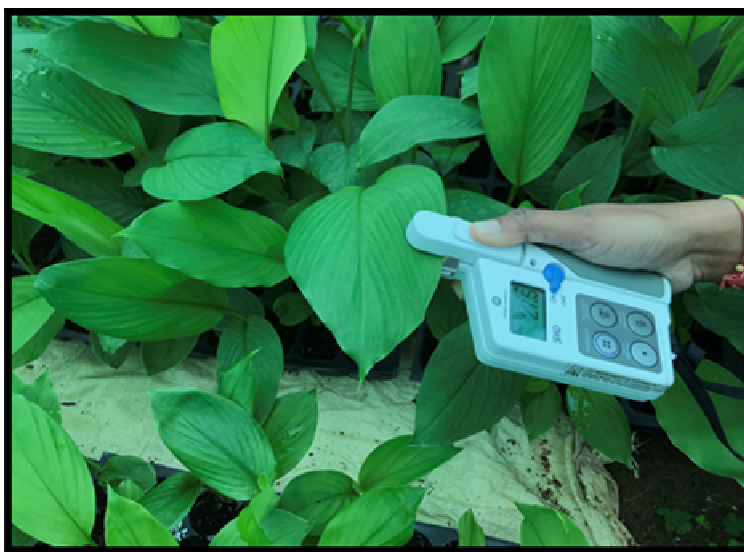
Plate 4 : SPAD meter reading – chlorophyll content
